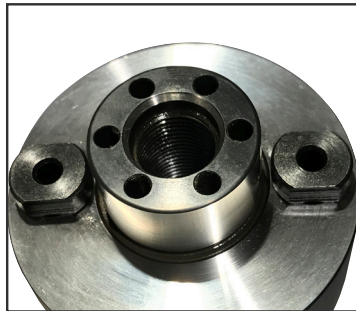
6 coolant ports for maximum pressure
